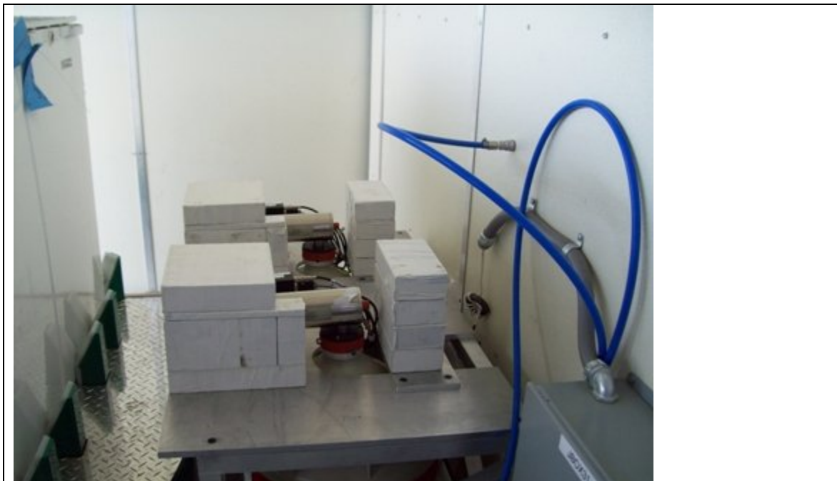
Figure 2: HPGE configuration for the Los Alamos SHENC.
