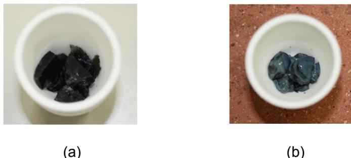
Fig. 2. Photographic images of glass specimen 6 (a) before and (b) after phase separation
