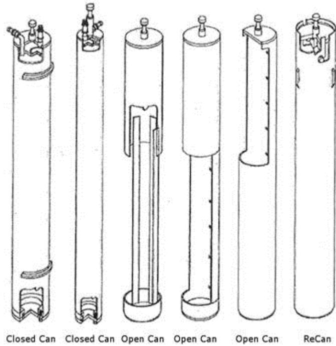
**Figure 2 Schematic of the Different Fuel Can Designs used at CRL**
