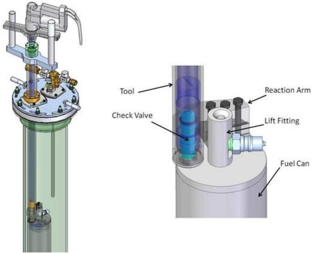
**Figure 4 Schematic of Check Valve Removal Equipment**
