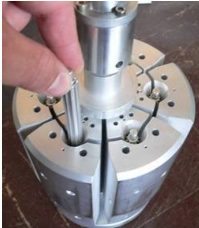
Figure 4 Target Holder in Free State with Receiving Holes Providing Clearance for the Targets
