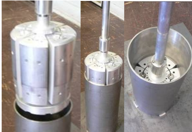
Figure 5 Target Holder Inserted into a Representative Cask Cavity
