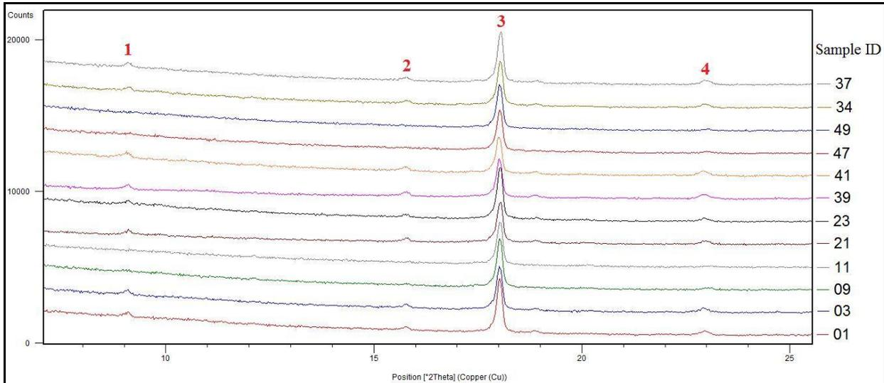
Fig. 3 – Close-up of the 7° to 26° range of the diffractograms of the 12 cement paste samples
