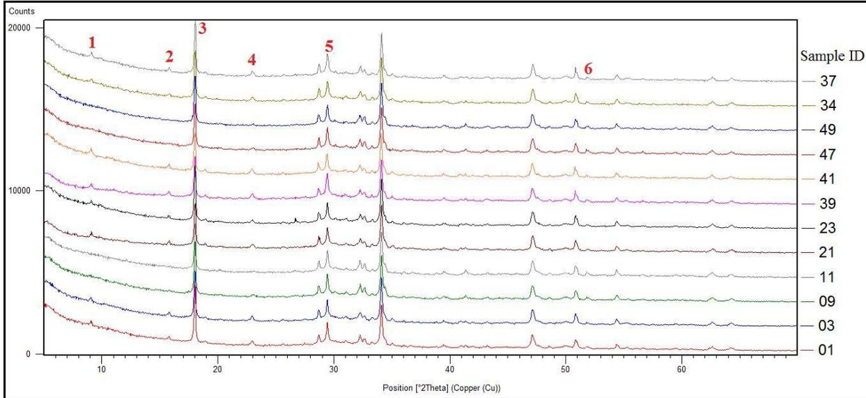
Fig. 2 - Diffractograms of 12 cement paste samples.
