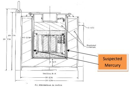
Figure 8 – Illustration of the Weather Bureau RTG with Mercury
