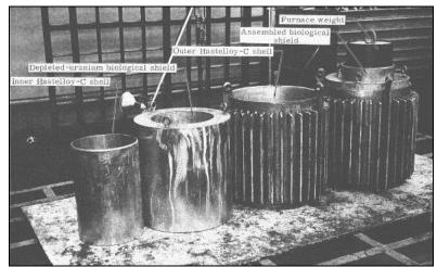
Figure 9 – SNAP-7C RTG current configuration
