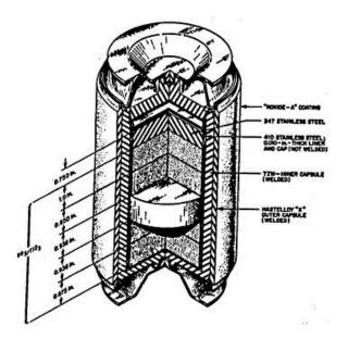
Figure 2 – Typical Configuration of an RTG Fuel Source
