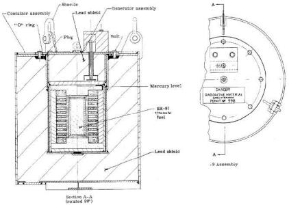
Figure 5 – Schematic of the Weather Bureau and SNAP-7C RTG
