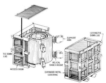
Figure 7 – Illustration of the BUP-500 RTG in its Present Container
