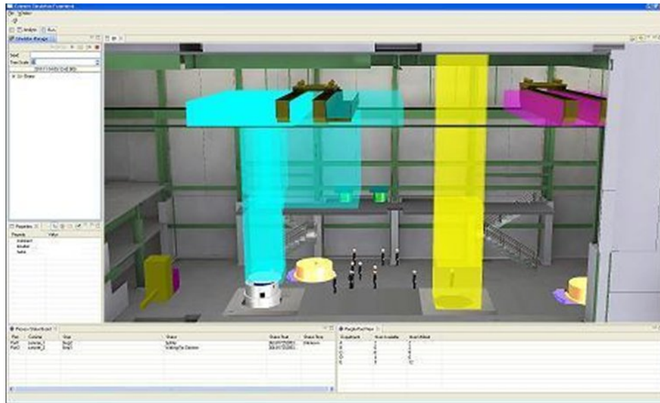
Fig 2: Model visualization of a facility with Smart Crane path planning
