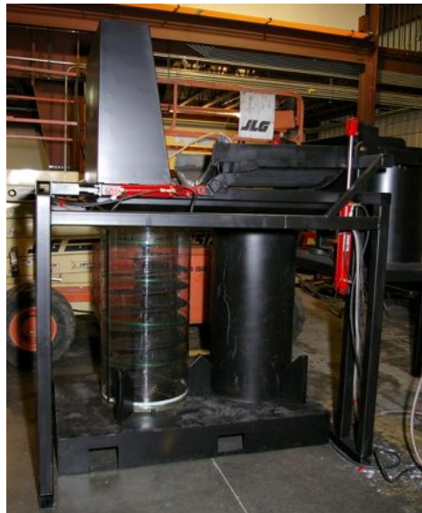
Figure 5 - Trialling of Pile 1 Helical Waste Liner
