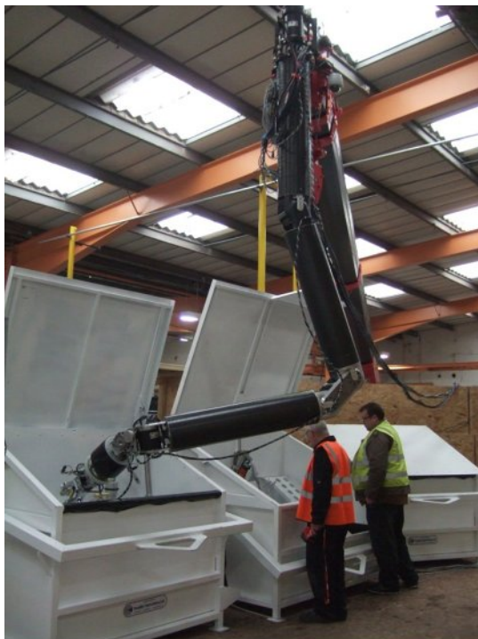
Fig 1: Powered Remote Manipulator Mounted to Spider Crane
