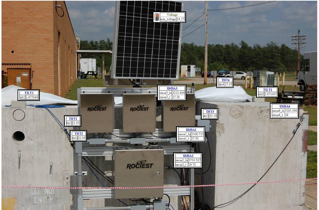
Figure 1. Prototype of the dashboard which can be used to display user specified data
