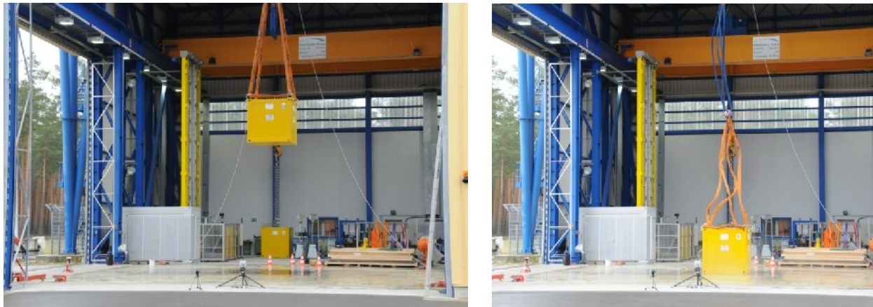
Fig 2. 5 m drop test on a Konrad Type II steel sheet container (EWB/GNS) onto the unyielding IAEA foundation of the BAM drop test facility on its Test Site Technical Safety (TTS).
