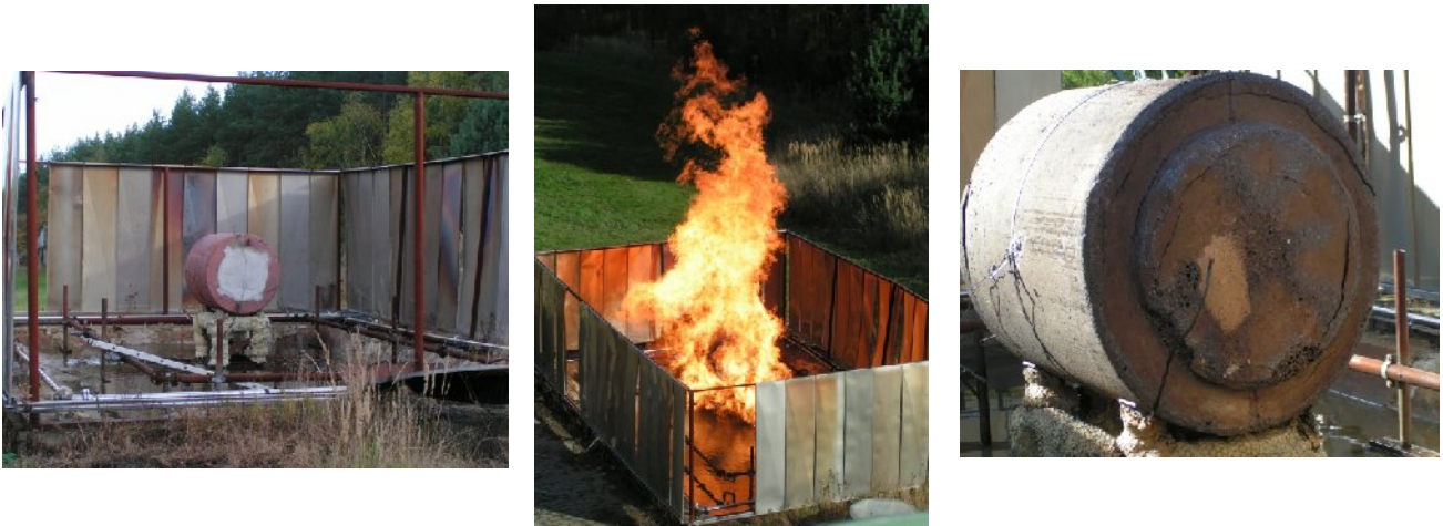
Fig 1. Disposal fire test scenario (800°C, 1 hour) on a round Konrad concrete container containing a 200 liter drum.
