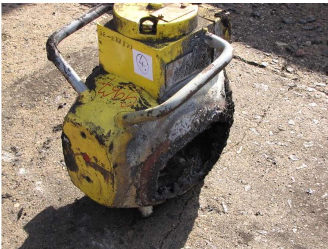
Fig. 3. Damaged level indicator with activity of 1.25 GBq of Co-60.
