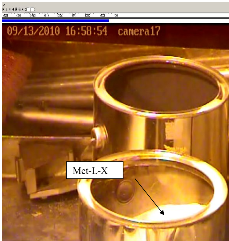
Figure 5. Daughter Can After Second Thermal Event with Met-L-X.
