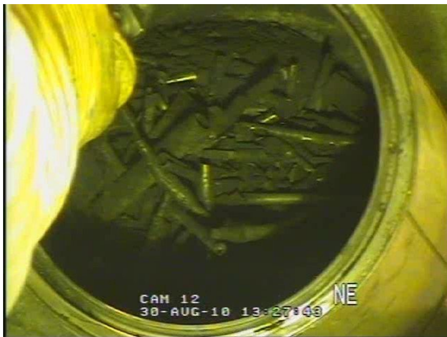
Figure 3. ANLE-11 Can #189 After Flames Extinguished with Met-L-X.
