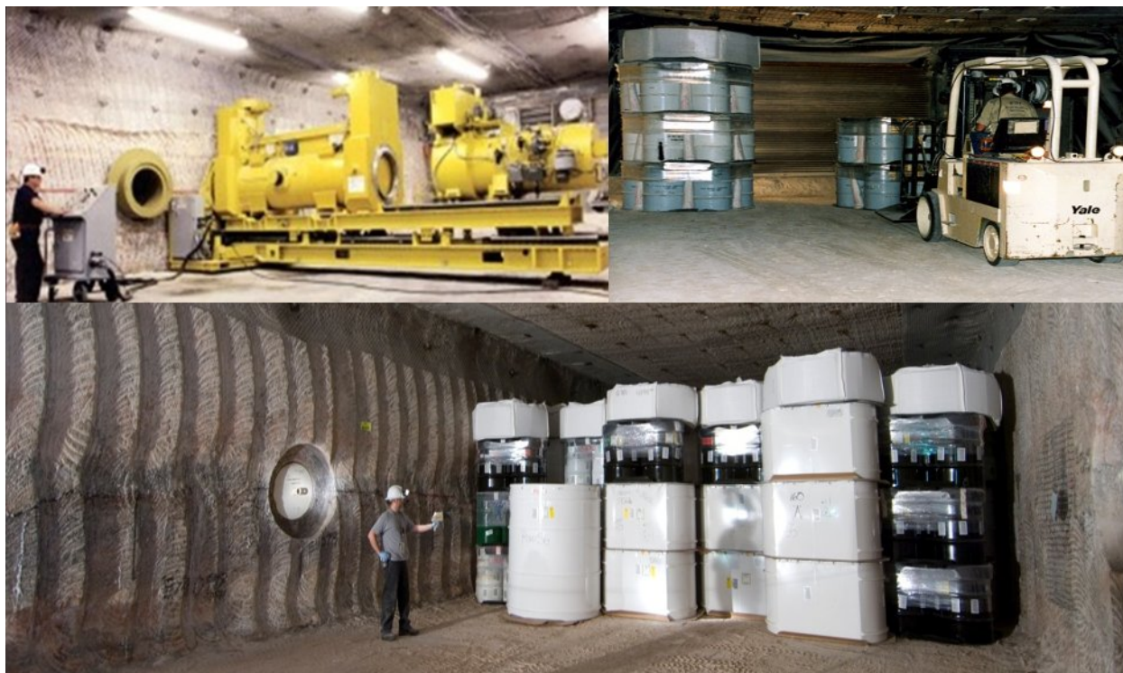
Fig. 5. Photos of equipment used for emplacing RH-TRUW (left top photo) and CH-TRUW (top right photo) and a portion of a disposal room with emplaced TRUW (bottom photo).
