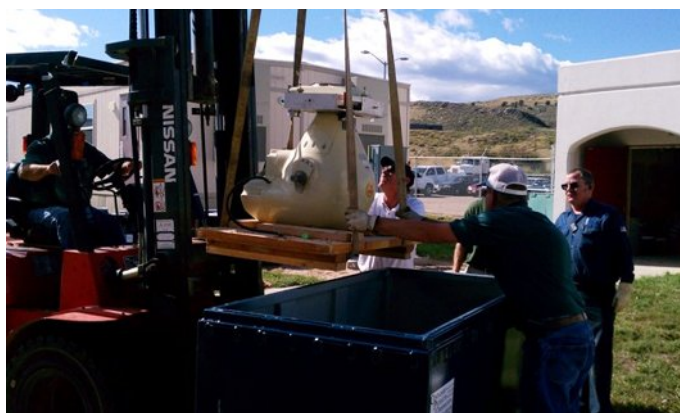
Fig. 1. Loading of the sources into a custom Type 7A container.
