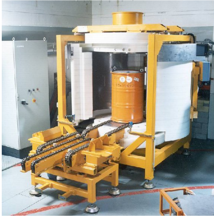
Fig. 4 FEMOS monitor for measuring of waste drums
