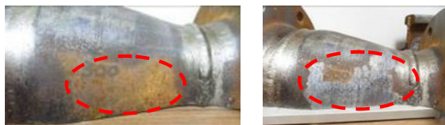
Fig. 1. Ablation of iron oxide (Before treatment (Left), After treatment (Right)).
