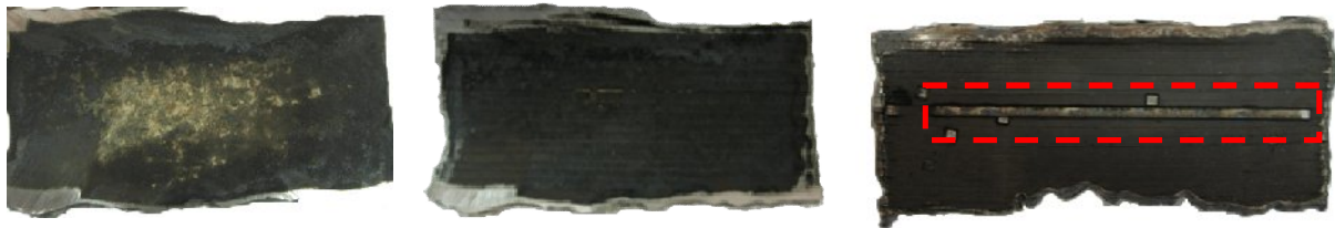
Fig. 3: Sample before ablation (Left), Sample after partial ablation (Center), Sample after complete ablation on one part (Right).
