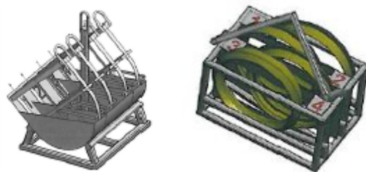
Fig 9. Racks for temporary buffer storage of bottom plates and upper flanges
