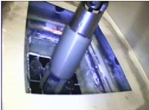
Fig 9. Retrieval of the first slug with a gripper
