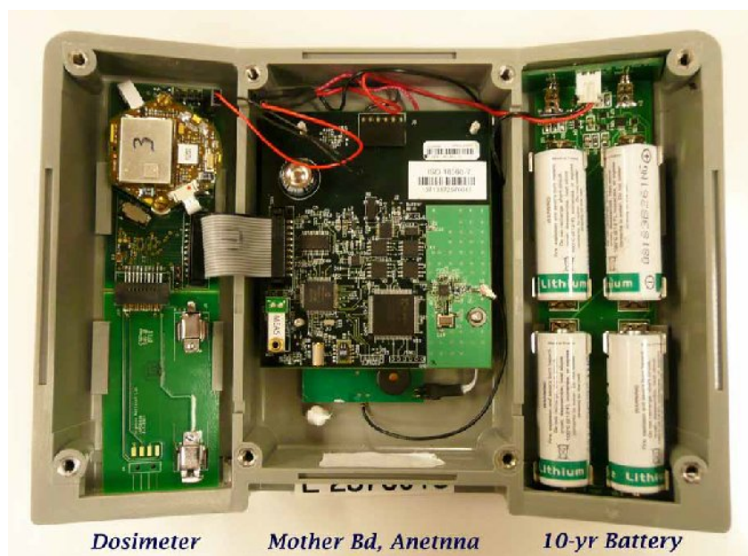
Fig. 1. Interior view of ARG-US RFID tags, with the metal back plate and seal sensor removed
