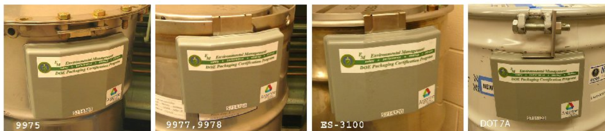
Fig. 2. Versatile form factor, which allows ARG-US RFID tags to be mounted on various types of drums
