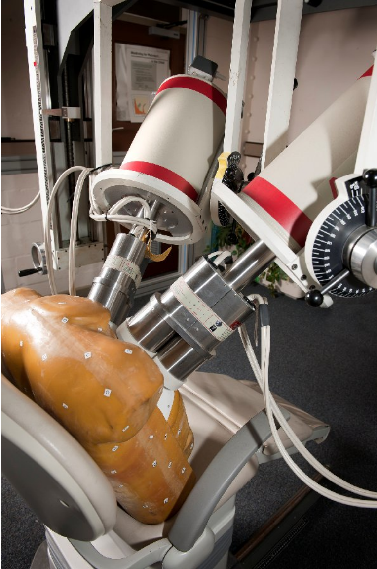
Figure 5 IVM monitor counting a calibration phantom
