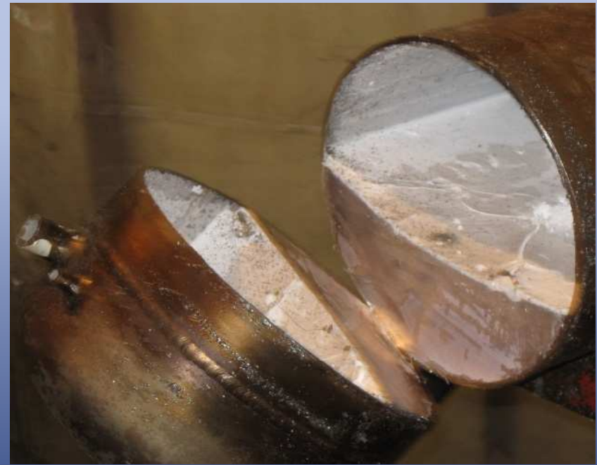
Sodium-filled interior of sealed vessel
