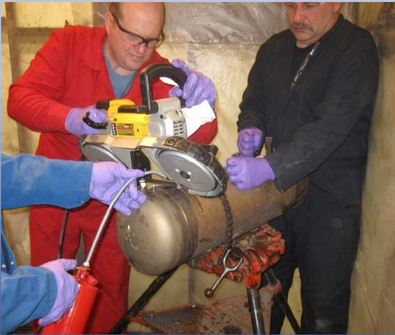
Accessing a sealed vessel containing Sodium
