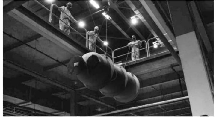
*An overhead crane lifts a large converter weighing several tons from a cell in the X-326 Process Building.*
