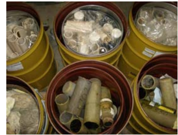
Figure 9 Example of overpacking and excessive pre-package effort
