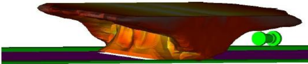
Figure 7 Fire surface temperature contour 10 seconds after the beginning of a simulation with a package in the tunnel at Z = 40 m. The fire surfaces in this figure are at the tunnel ceiling, wall, and at locations where the products of combustion mass fraction is 0.07.
