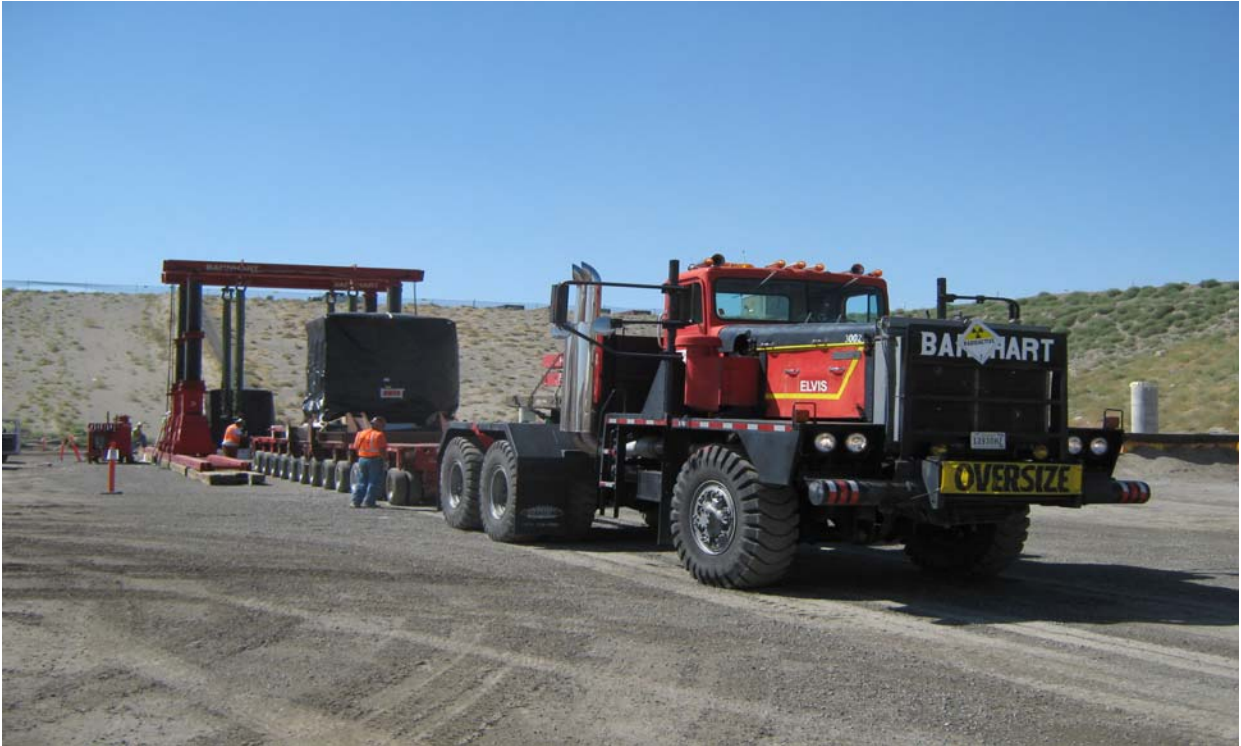
Figure 4. Packaged Hot Cell on Transporter at ERDF
