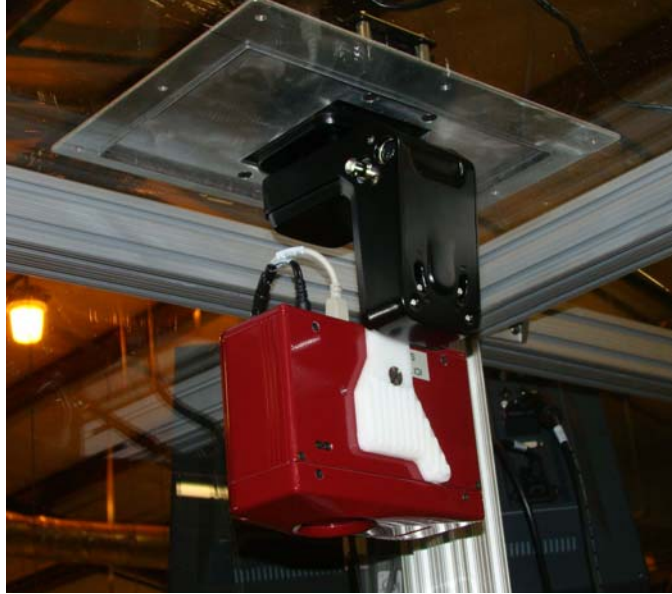
Figure 1 - ICI 7640S Infrared Camera Mounted to Pan and Tilt Unit
