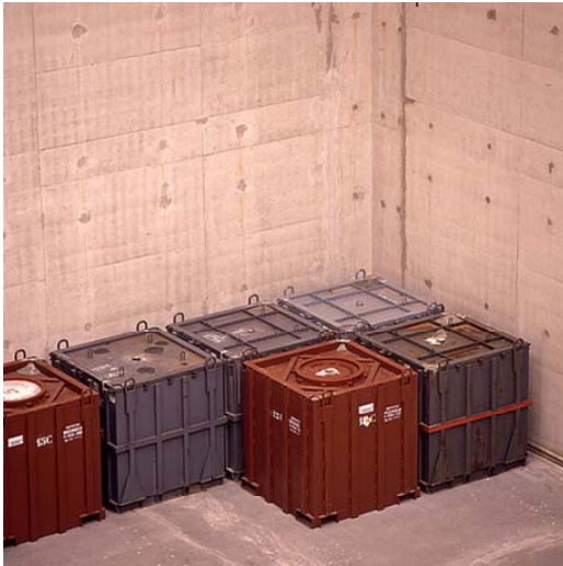
Figure 8: metallic waste package at Centre de l'Aube disposal facility (LIL-SL)
