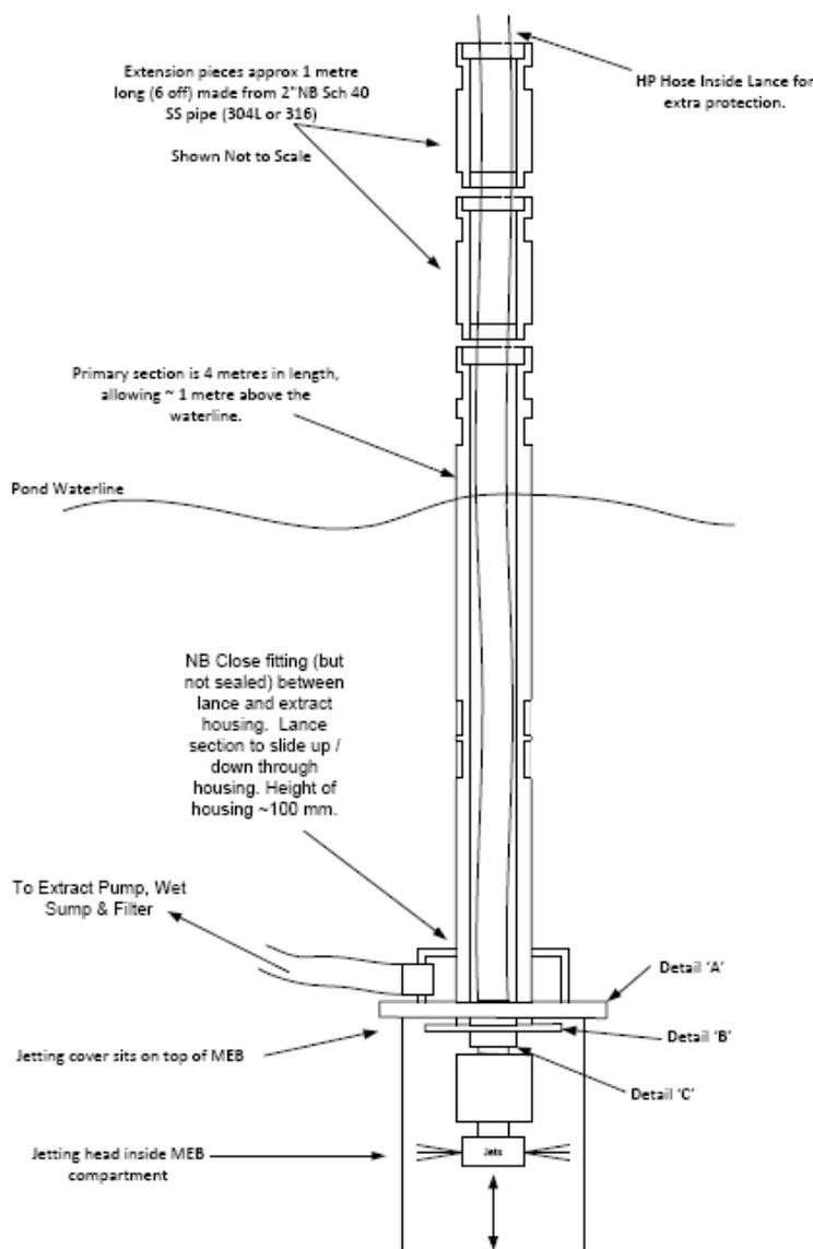
The lance assembly (Fig. 4) was connected to the building crane via dedicated brackets enabling the lance to be located on the top of each MEB compartment, then lowered and raised in turn. The lance moved freely through the sealed penetration of the main lance housing.
