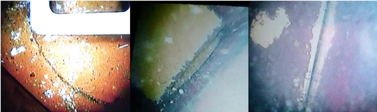
Fig. 6 - Crud layers in a) Type A MEB, b) top layer of Type B & c) lower layer in Type B
