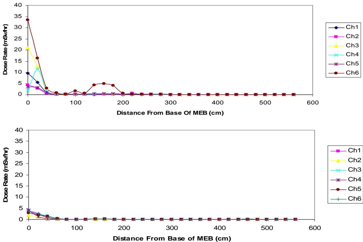
Fig. 3 - Typical MEBRAM profiles before and after decontamination.
