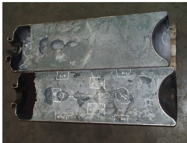
Figure 4. Location of UMo glass samples taken along a vertical cross section of the canister
