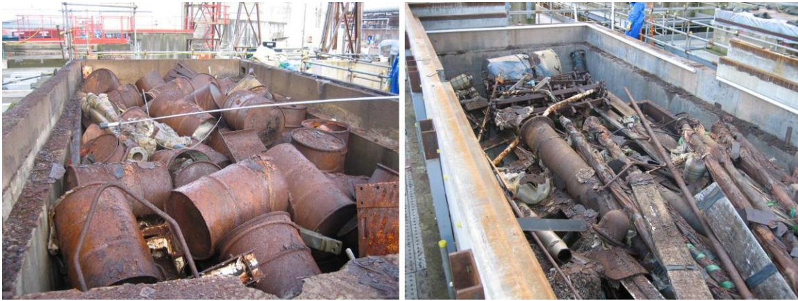
Fig. 1. Typical contents of the concrete storage cells filled with Low and Intermediate Level Wastes.
