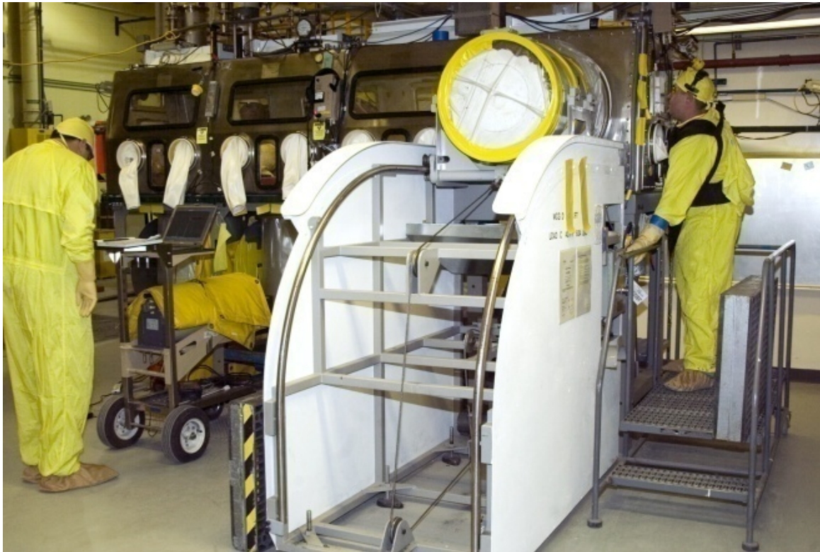
Fig. 3. Waste Characterization Glovebox in the LANL WCRR Facility
