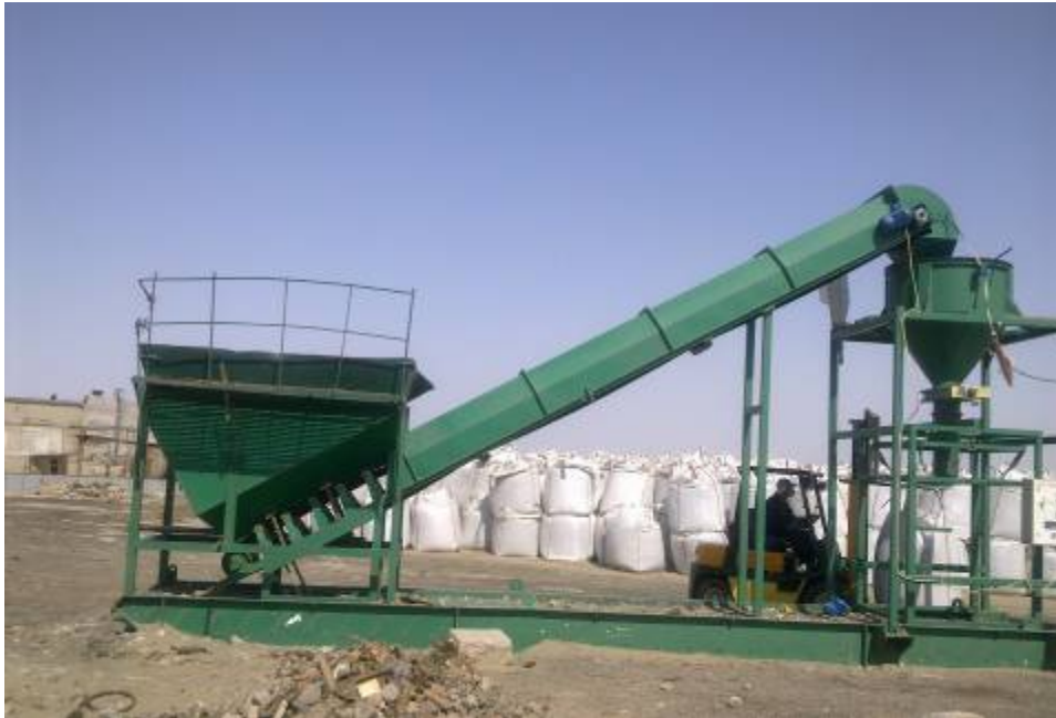
Fig. 5. Big-Bags' filling station
