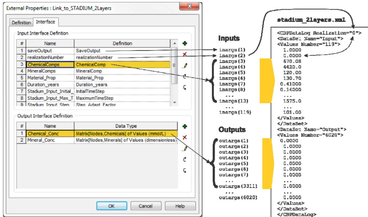
Fig. 2. Example of the GoldSim External Link Properties Interface and Corresponding Log File
