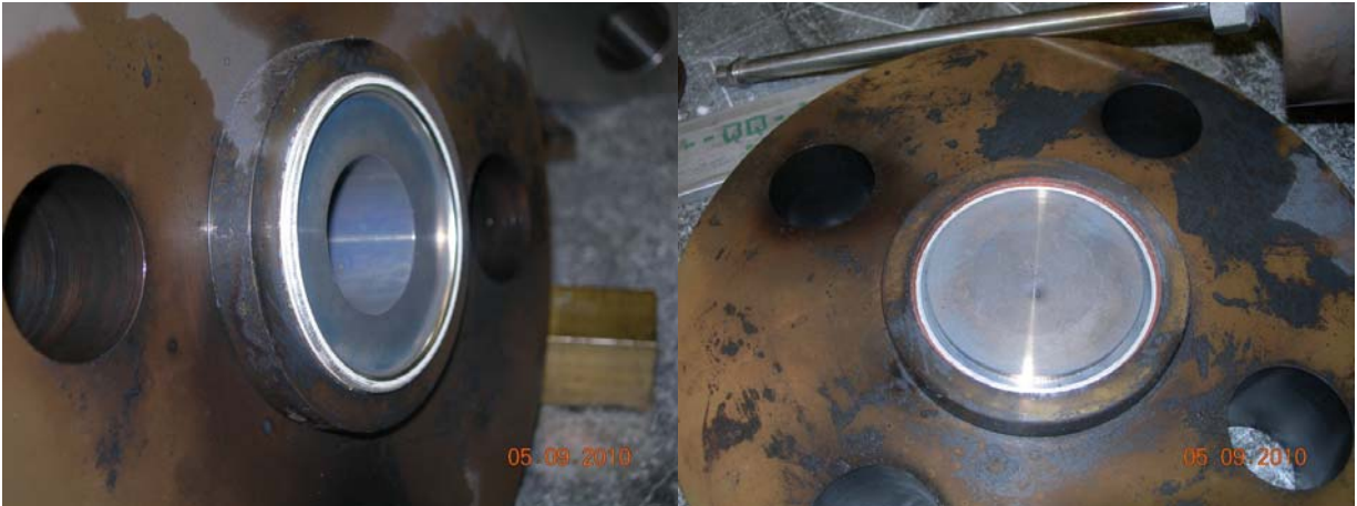
Figure 3: Postmortem photographs showing the O-ring bonded to the tested vessel body (left) and showing silver from the metallic O-ring deposited on the O-ring groove (right)
