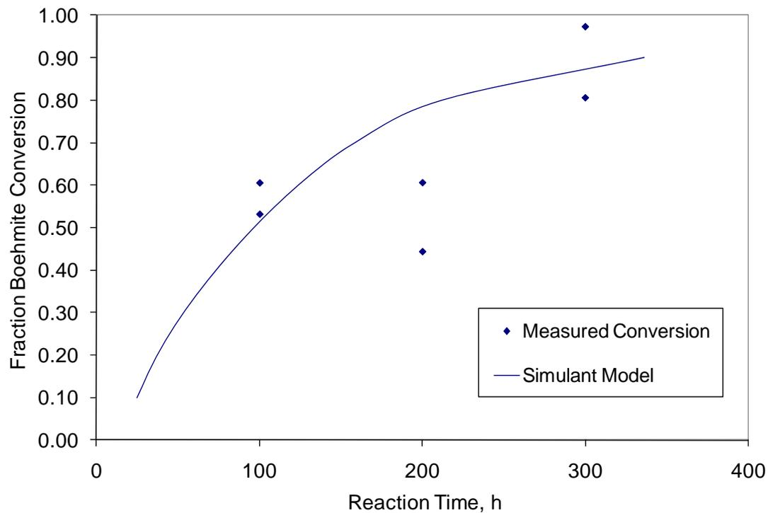
**Figure 1.** APYRAL AOH20 Boehmite Dissolution at 100° C
