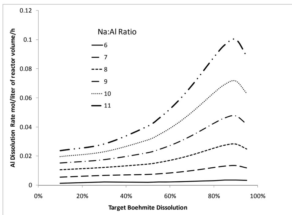
**Figure 2.** Aluminum dissolution per liter of reactor volume.
