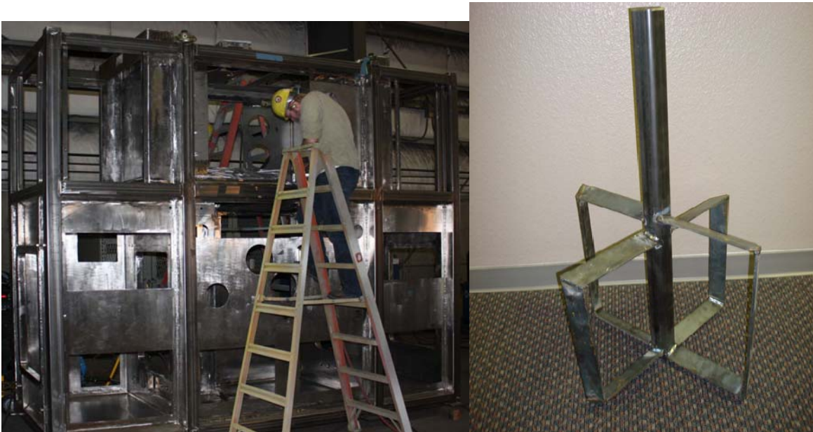
Fig 7: a) A GCMS Glovebox Being Fabricated, b) Developed GCMS D-paddle
