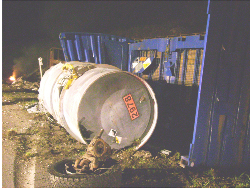
Figure 4 - The Type B cask carrying the UF6 did not leak, but carved a small trench in the interstate concrete, as shown in the bottom left corner of the picture.
