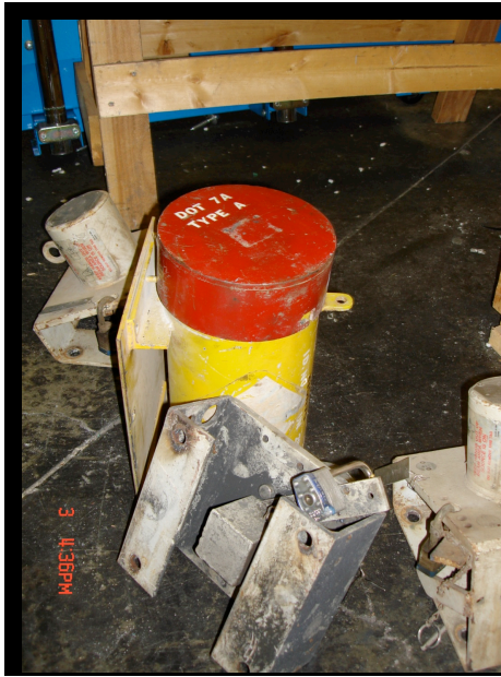
Figure 1 - Covering sources with shielding caused a Bremsstrahlung effect, resulting in increased radiation rates in the facility.
