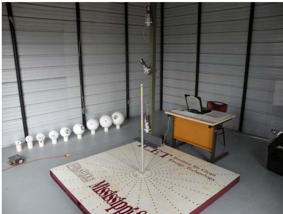
Fig. 1. Test stand used to create characterized radiation fields with a Cs-137 source placed 1 cm above the test stand. \text{LaBr}_3(\text{Ce}) detectors are located in the horizontal plane of the source and 1 m above and below the source.
