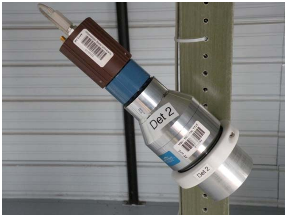
Fig. 3. LaBr 3 (Ce) detector mounted with an ORTEC ® digiBASE™.
