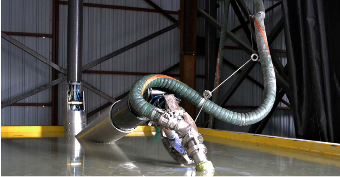
Figure 1 - RDA during factory acceptance testing, using a bulk suction tool to remove simulated tank effluent
