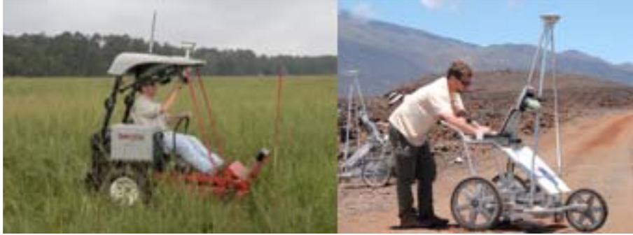
Figure 2. Photos of two survey platforms used by the MSU ICET survey system. The right photo is a motorized platform equipped with a single 10 x 10 x 40 cm (4 x 4 x 16") NaI(Tl) and four 7.6 x 7.6 (3 x 3") LaBr<sub>3</sub>(Ce) detectors. The right photo shows a man-portable three wheeled cart equipped with a single 17.8 x 17.8 (7 x 7") NaI(Tl) and two 7.6 x 7.6 (3 x 3") LaBr<sub>3</sub>(Ce) detectors. Both platforms have on-board computers and GPS systems.
