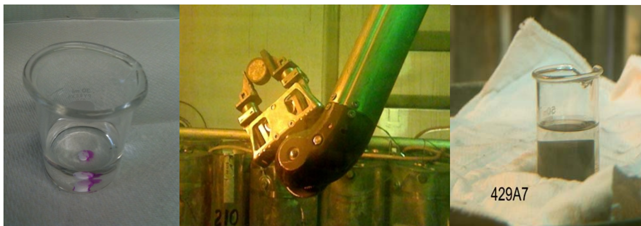
Fig. 1. From left to right: A sodium hydroxide tablet submerged in the ethanol/phenolphthalein indicator showing the positive pink color indicative of the ethanol-sodium reaction; a met mount disk held in a remote manipulator hand inside the hot cell; a met mount submerged in the ethanol/phenolphthalein solution inside the hot cell showing no evidence of an ethanol-sodium reaction (no pink color and no hydrogen gas bubbles).
