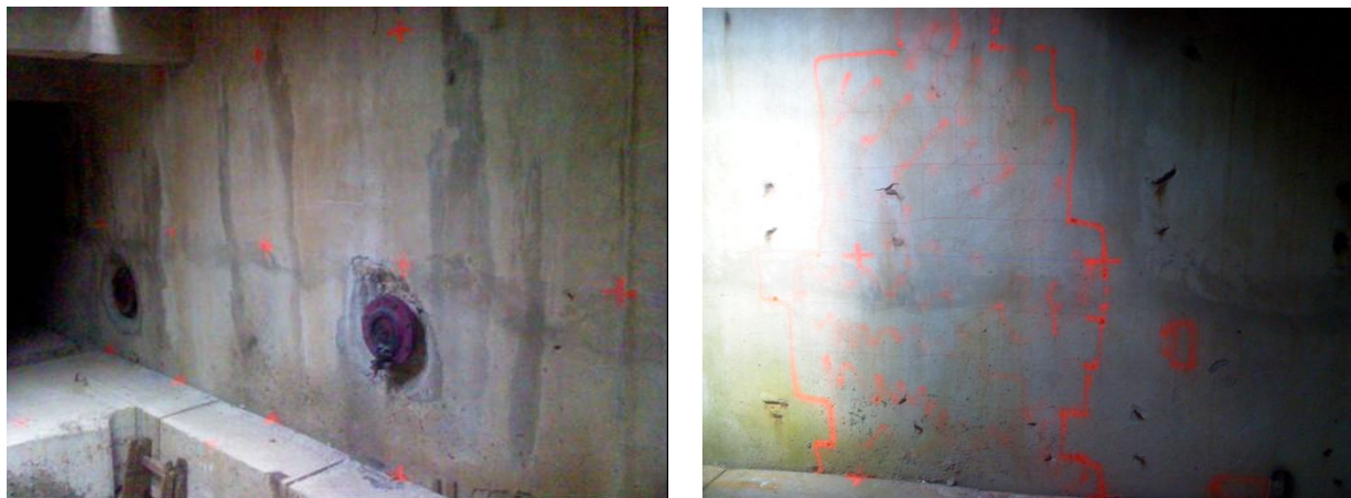
Fig.1 Example of monitoring grid and place with measured values above the clearance level.
