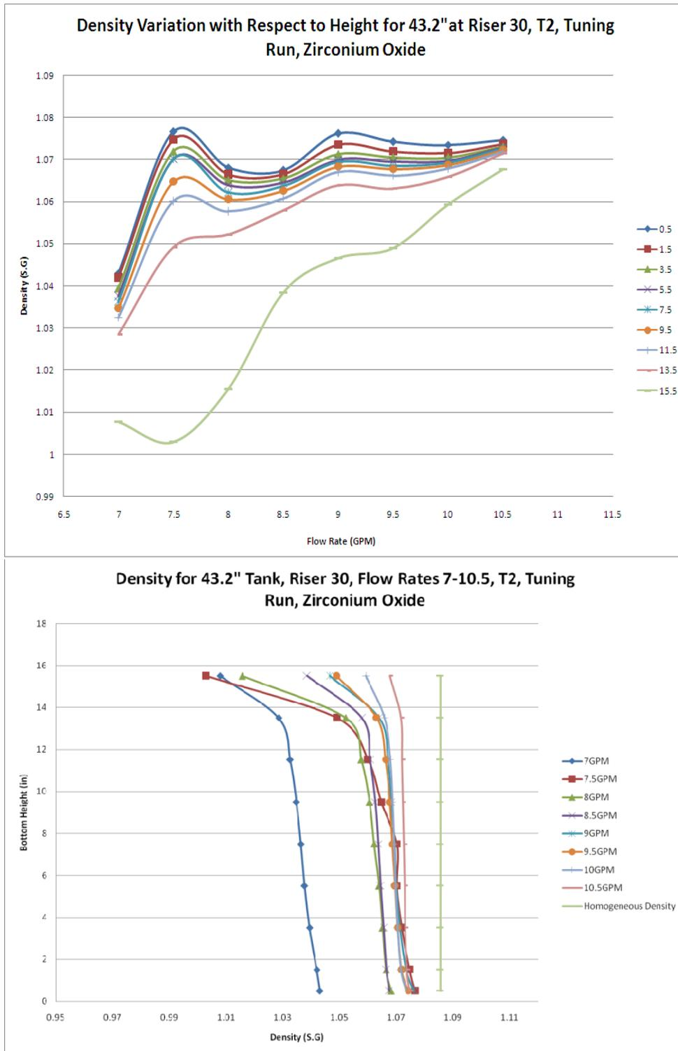
Fig. 2. Density vs. Location Plots in 110 cm Dia. Mixing Test Vessel
