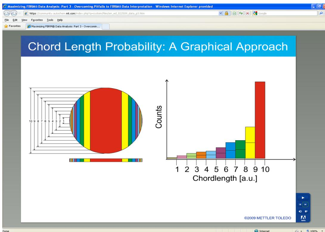
Fig. 3. FBRM® Chord Length Distribution for a Single Particle
