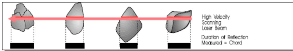
Fig. 6. Duration of Reflected Measurement Equate to Chord Length
