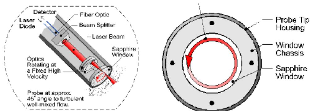
Fig. 5. Schematic of Mettler Toledo FBRM<sup>®</sup> Probe
