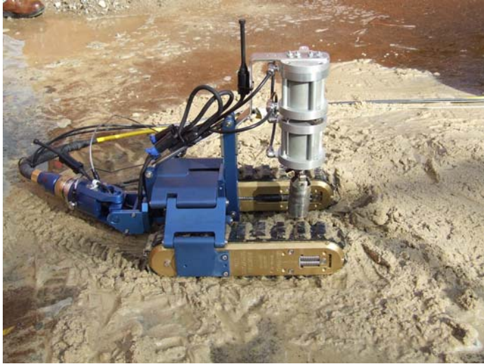
Fig. 2. Commercial crawler after sampling modifications
