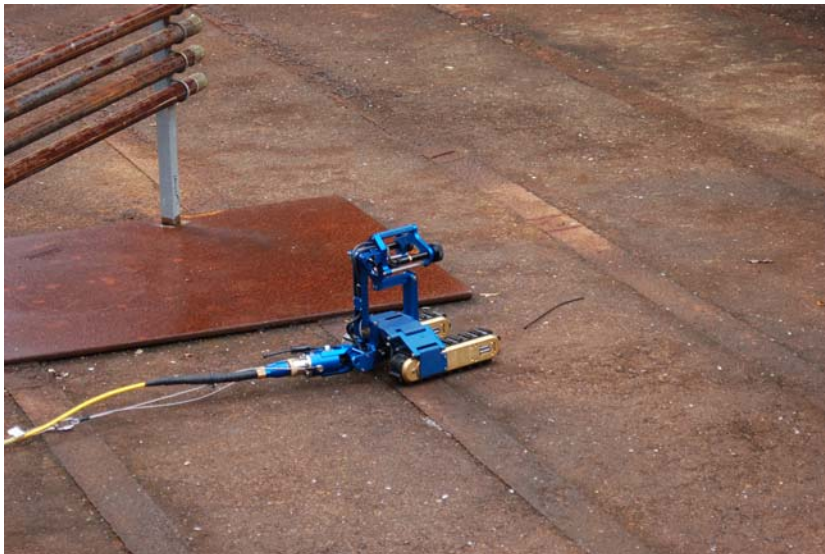
Fig. 1. Commercial inspection crawler
