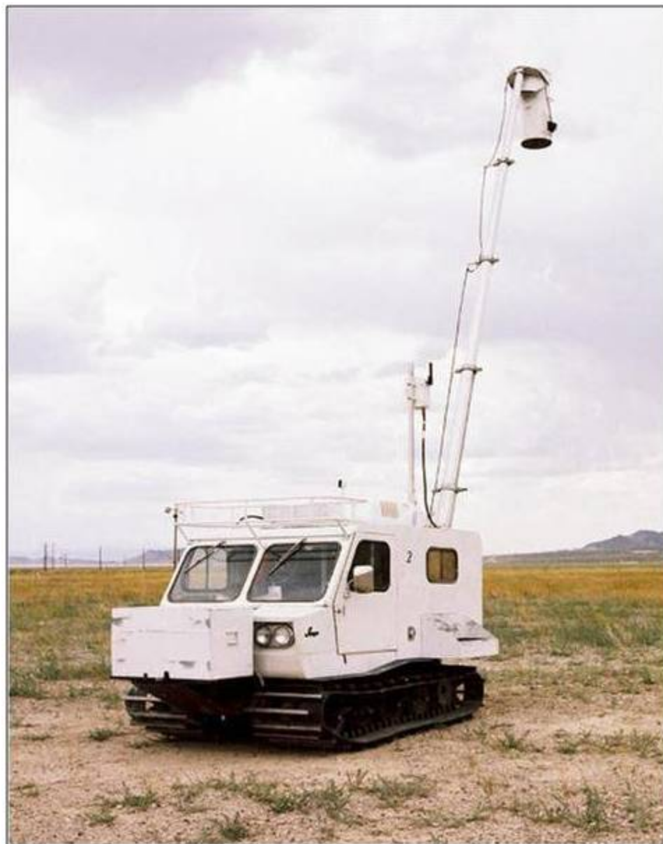
Fig 2. A tracked vehicle with a mast which was mounted with a high purity germanium detector for the RIDP measurements.
