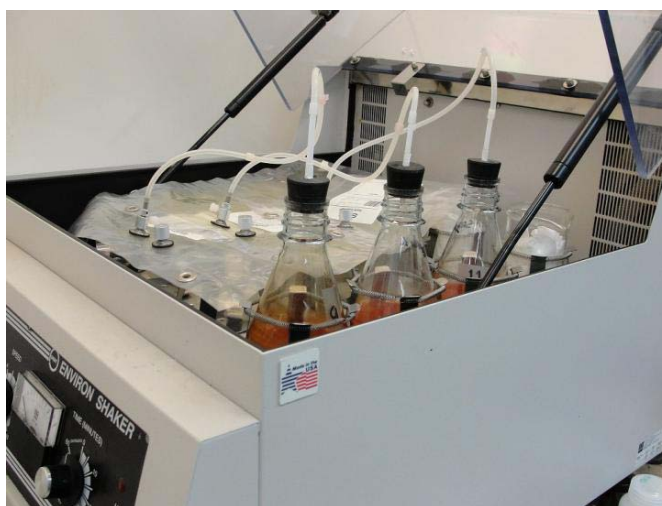
Fig. 1. Photograph of shaker, flasks and Tedlar bags
