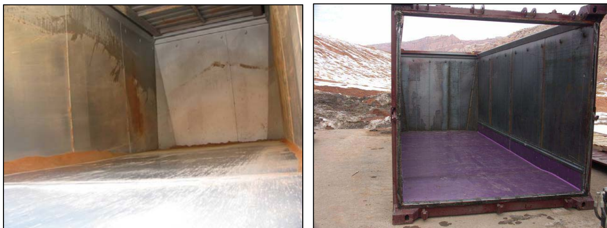
Fig. 3. Photographs of interiors of containers with a sprayed-on liner (left) and panel liner (right).
