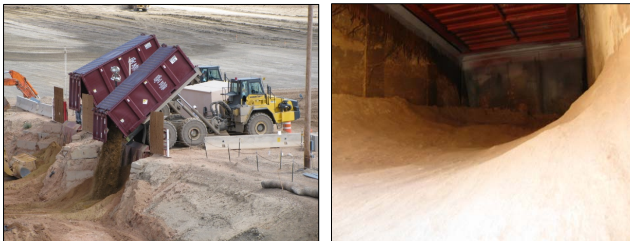
Fig. 1. Photographs of RRM being emptied from a container (left) and the holdup after emptying (right).
