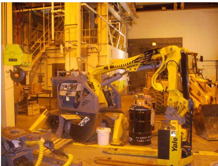
Fig. 1. Spare BROKK 330 being modified for remote operation within the VF.
