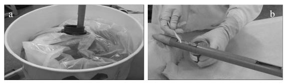
Figure 1 – Sampling of ion exchange resins: (a) thief sampler being inserted in the plastic bag that contains the waste; and (b) sample in the lower sampling port being transferred to a sample container.
